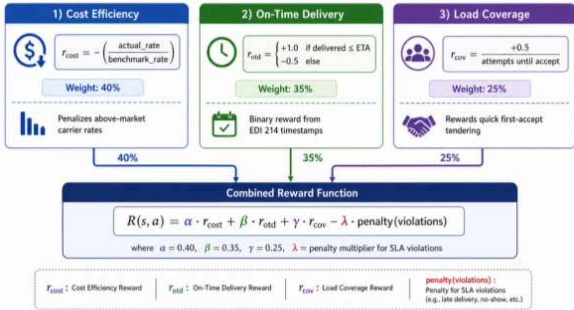
Figure 3. Multi-objective reward function decomposition for the RL tendering agent. The combined reward R(s,a) balances freight cost efficiency (40%), on-time delivery (35%), and load coverage (25%), with an additional SLA violation penalty term.
