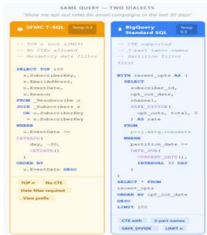
Fig. 3. Dialect-specific SQL generation for the same natural language query in SFMC T-SQL (left) and BigQuery Standard SQL (right).
