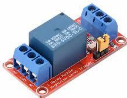
FIGURE: 3.1.7 Relay model to control switches
